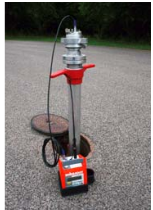
PAM HYDRO-2 connected to a P-2 correlator transmitter
